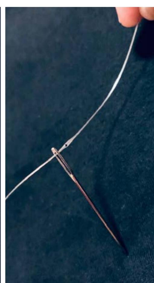
feel any different from a regular one; the fibre is unnoticeable because of its flexibility and lightweight. The fibre and its elements are similar to the data storage in computers. You can turn on an individual element without turning on the complete chain of the elements in the fibre.
